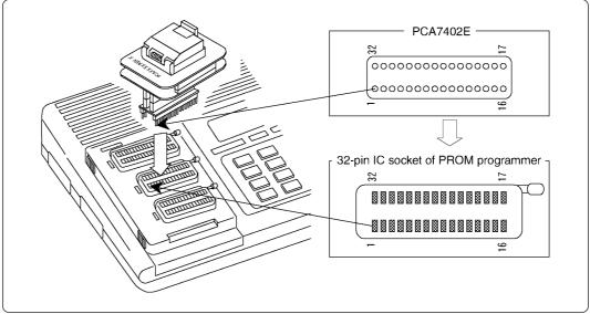
Figure 4.1 Attaching the adapter to the PROM programmer
